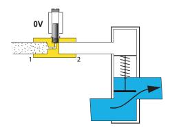
Here, there is no tension though the spool and the solenoid valve is held down by the force of the spring. This is so that no compressed air reaches the water valve's piston. The water valve is now open, which is its position unaffected by compressed air.
