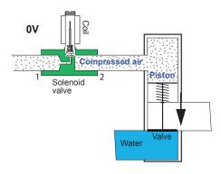
Here, there is no tension though the spool and the solenoid valve is held up by the force of the spring. This means that compressed air affects the water valve's piston and the water valve closes.
