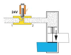
Now, the spool is fed with voltage which means that the solenoid valve opens and compressed air reaches the water valve's piston. The water valve is then pusched down and closes the water flow.
