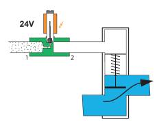
Now, the spool is fed with voltage which means that the solenoid valve closes and no compressed air reaches the water valve's piston. The water valve is now open, which is its position unaffected by compressed air.
