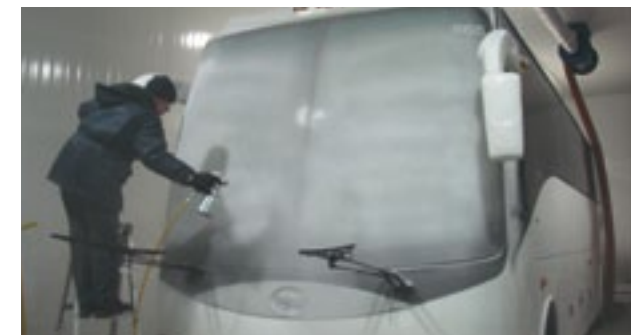
Layer of frost applied to windscreen for Defrosting Test.
