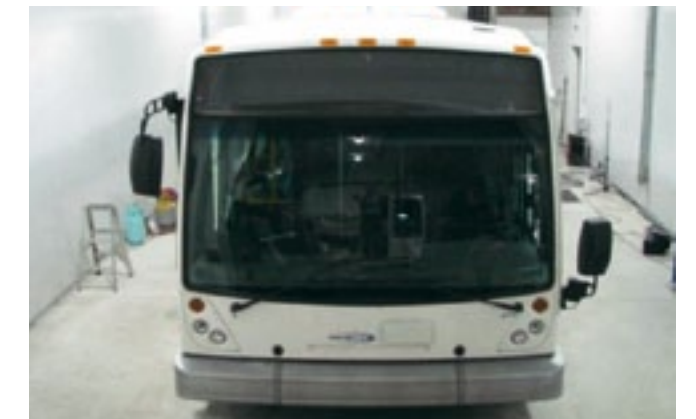
Transit bus in Large Chamber ready for A/C system test.
