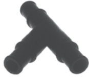
27-0102 Y-splicer 5/8" 43% fibreglass reinforced nylon 6/12. For 5/8 and 3/4" hose.
