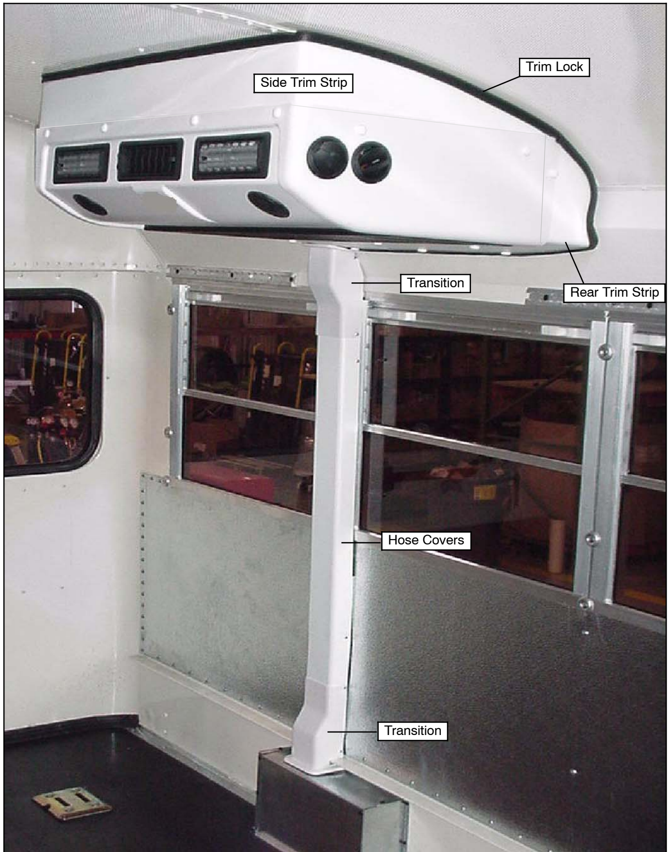
Figure 2-27 EM-2 (Gen V) Side-Mount - Free Blow, Installed (Complete)
