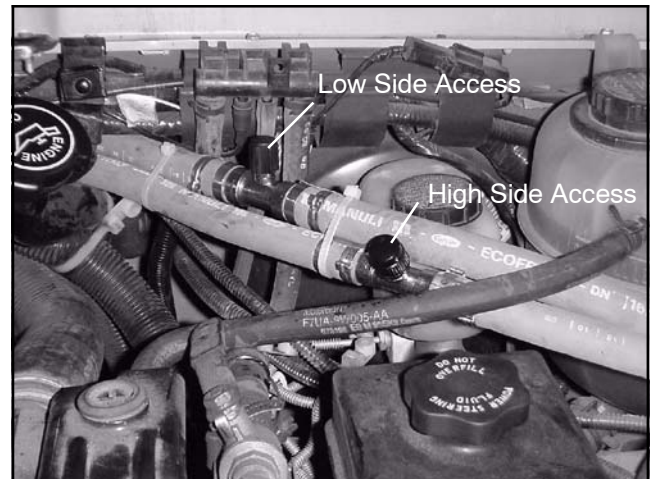
Figure 4-24 Engine Routing (With High & Low In-Line Access Fittings)
