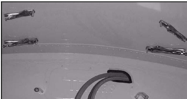
Figure 2-8 Locking Pliers Clamped to Carriage Bolts
