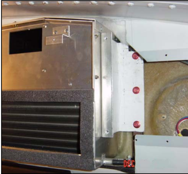
Figure 2-60 IW-1 Secured To Structure Rail TBB
