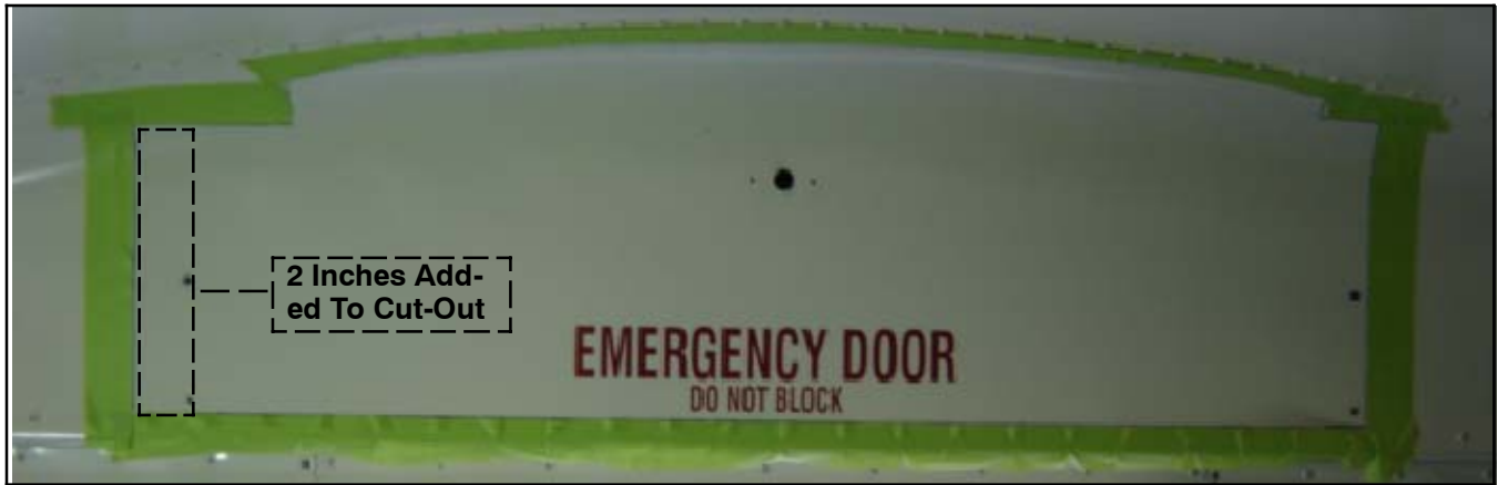
Figure 2-37 In-Wall Marked For Cut-Out
