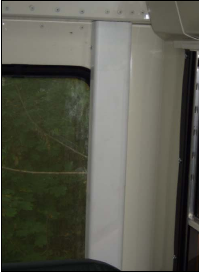
Figure 4-13 Correct Hose/Harness Corner Routing (Window Not Blocked)
