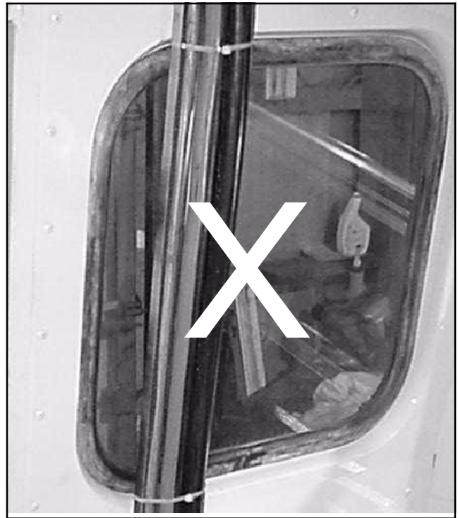
Figure 4-12 Incorrect Hose/Harness Routing Rear window is partially blocked.
