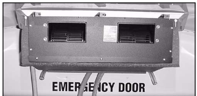
Figure 2-10 Evaporator Mounted to Flat Ceiling
