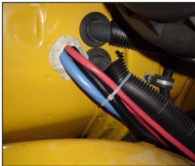
Figure 5-8 Electrical Control Cables Thru Fire Wall To Electrical Control Panel
