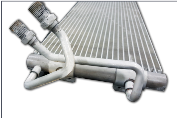
MCC coil after SWAAT* testing
